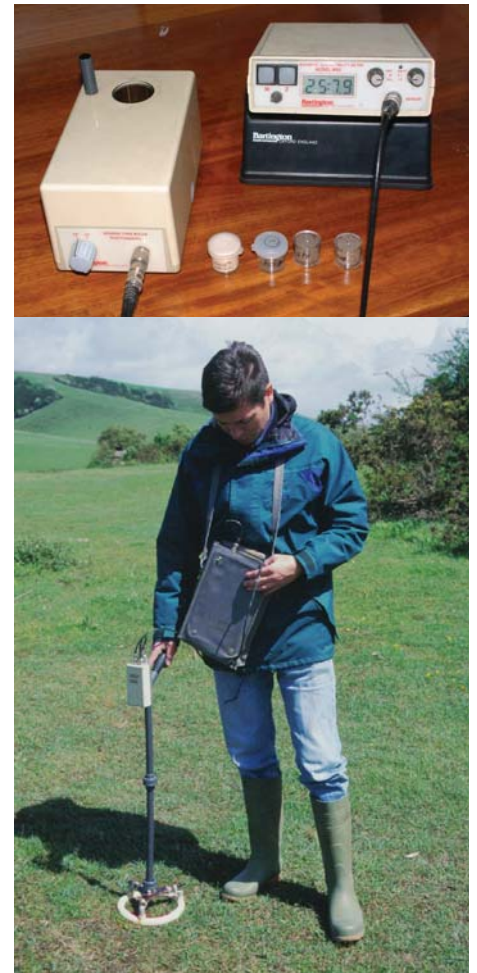
Fig 20 (below) Area magnetic susceptibility survey (a) showing increased response over an area of dense magnetometer anomalies (b). Low responses to the NE correlate with recent soil dumping, but some finer detail is not represented, such as a cemetery (c). Fig 21 (above) Bartington MS2 magnetic susceptibility meter in use: (a) in the laboratory with collected 10g soil samples and; (b) on site with a field coil.
