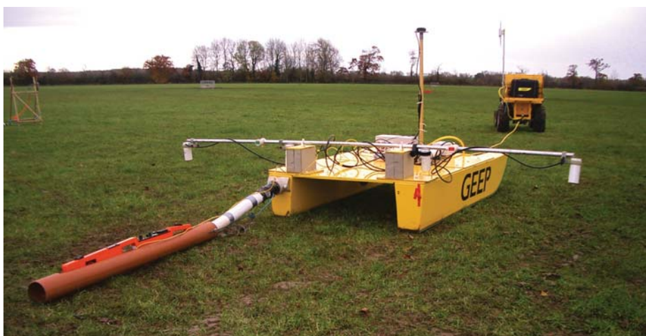
Fig 1 (above) The GEEP towed mobile sensor platform with built-in GPS (photograph courtesy of Ian Hill, University of Leicester).
