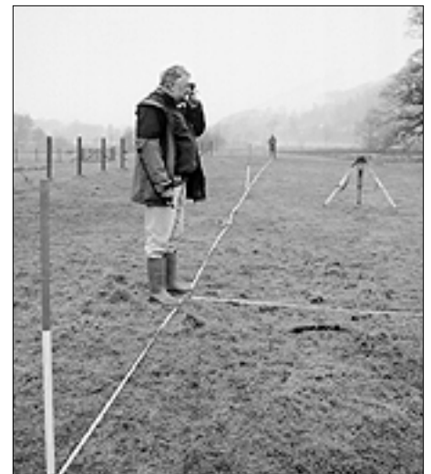
Figure 4 The optical square in use, raising a long offset from a tape line.
