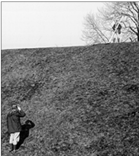
Figure 19 Measuring a substantial scarp with the pocket level: the observer’s eye height (1.6m) multiplied by the number of observations taken (3), minus the reading on the staff at the last observation (0.3m) gives the height of the scarp (4.5m)
