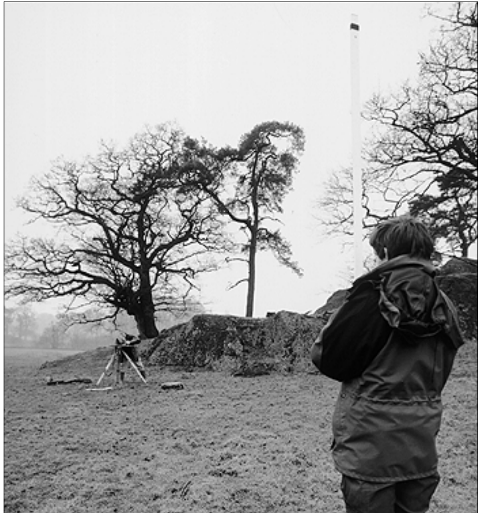
Figure 13 The plane table: observing a point of detail.
