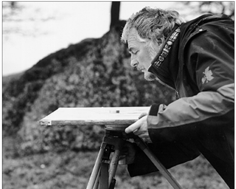
Figure 11 Levelling the plane table with a pond bubble.
