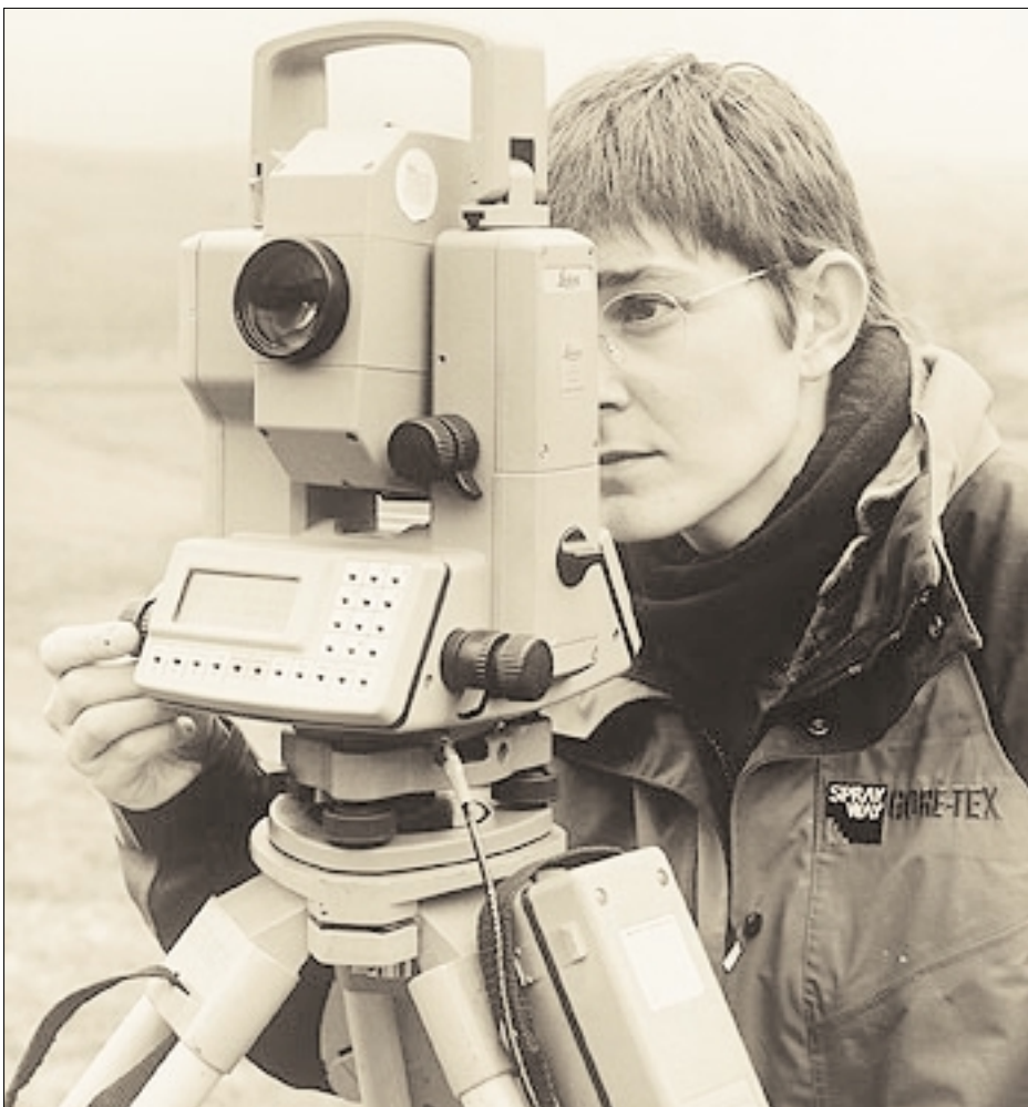
Figure 2 'Total station' EDM: electronic survey instruments supply control to a high degree or accuracy, but are not absolutely necessary for archaeological survey. Indeed, it is worth remembering that before the 1970s all survey was done without benefit of electronic instrumentation, to levels of accuracy far higher than those needed for archaeological earthwork survey.
