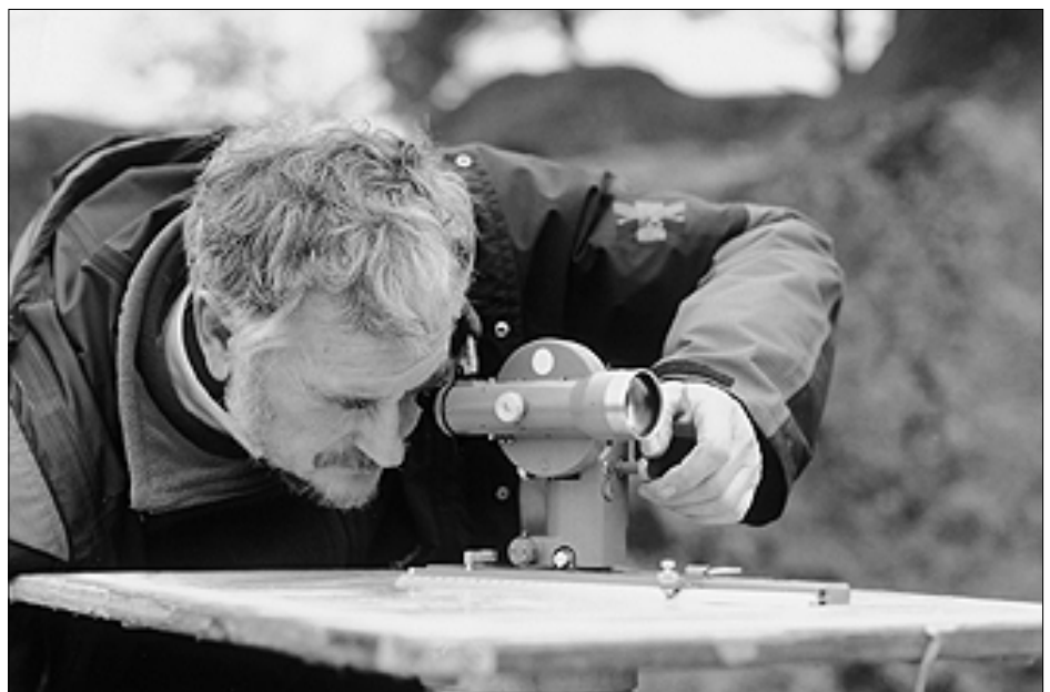
Figure 14 Observing with a self-reducing alidade: adjusting the vertical screw to bring the 'zero line' to zero.
