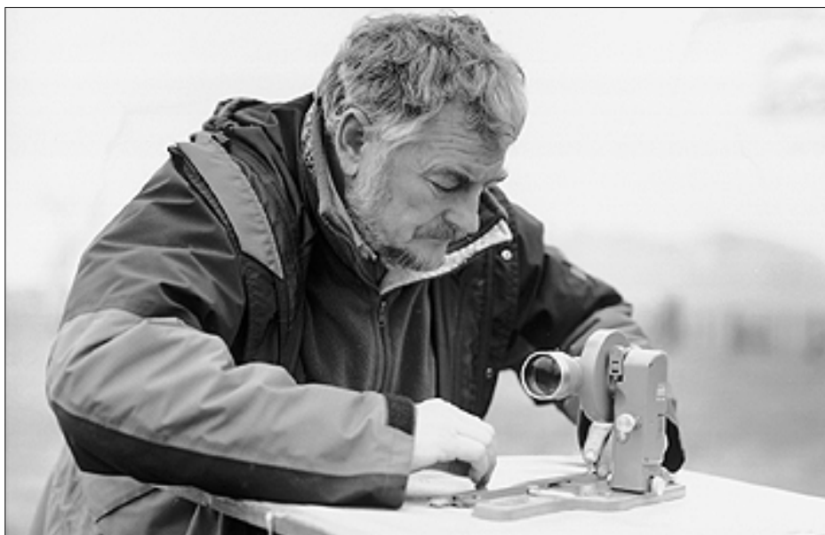
Figure 16 Pricking a point with a self-reducing alidade. Note that the observer has physically moved around the table to face the scale bar 'head on' and to avoid the danger of nudging the alidade by leaning across it.
