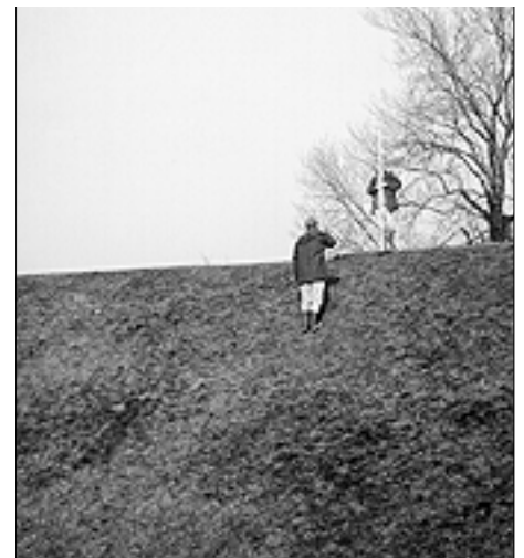
Figure 19 Measuring a substantial scarp with the pocket level: the observer’s eye height (1.6m) multiplied by the number of observations taken (3), minus the reading on the staff at the last observation (0.3m) gives the height of the scarp (4.5m)
